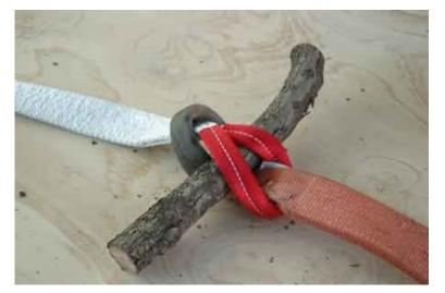
THIS IS AN ACCEPTABLE METHOD, but the stick will still do damage if one of the straps break.
