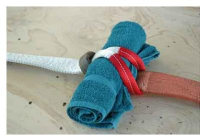
THIS IS THE RECOMMENDED METHOD, as the towel is not likely to cause too much damage if one of the straps break.
